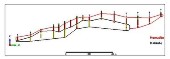
Image 4 - Vertical section 11 containing their respective holes and geological interpretations.
