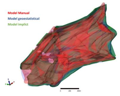
Image13- Overlapping models of itabirite litology.
