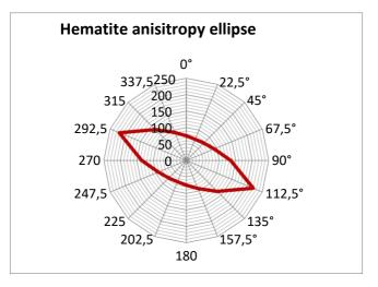
Image 7 - Continuity analysis graph for hematite mineralization.
