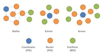
Figure 2 – Topologies that can be formed from RFD and FFD physical devices and Coordinator, Router, and End Point logical classes [5].
