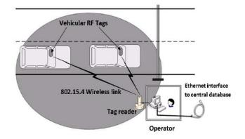
Figure 3 – Vehicular identification system using the 802.15.4 standard [6].
