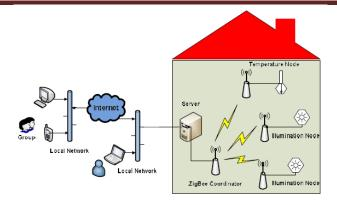
Figure 4 – Proposal of a residential automation using Zigbee [9].
