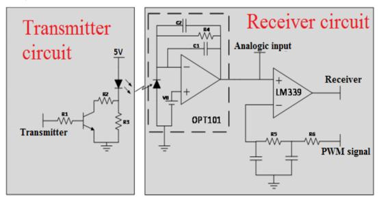
Figure 6 - Simplified circuit of the transmitter and receiver
