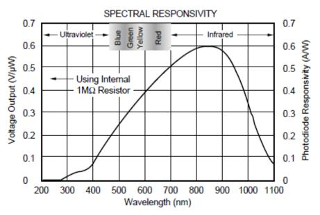
Figure 2 - Spectral responsivity of OPT101 (TEXAS INSTRUMENTS, 2003)
