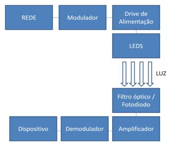
Figure 1 - Simplified Block Diagram of a VLC system
