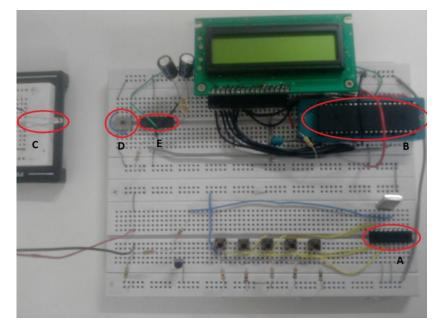
Figure 7 - Circuit mounted on the breadboard, where: A) PIC transmitter, B) PIC receiver C) Red LED D) Photodiode Amplifier E) LM339
