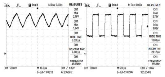
Figure 8 - Received by the photodiode signal with 50KHz and 1KHz
