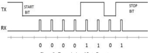
Figure 5 - Transmission of Data Format
