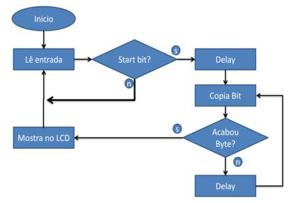
Figure 4 - Receiver flowchart
