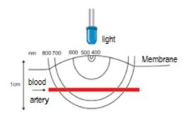
Figure 1. Light penetration into the skin as a function of wavelength [1].
