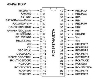
Figure 2.PIC16F877A microcontroller pinouts.
