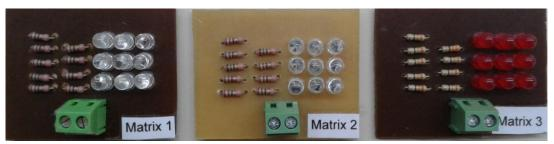
Figure 3. Three different matrixes forming a 3x3 LED matrix.
