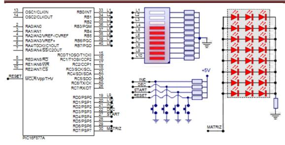
Figure 4. Electrical diagram of the second microcontroller system for the matrix of LED's.
