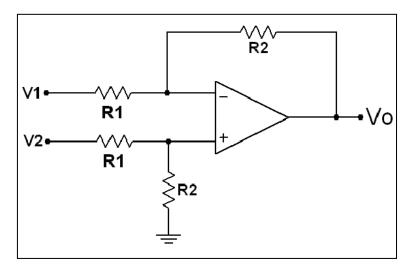
Figure 3. Circuit in subtractor configuration used in the development of signal suitability system.
