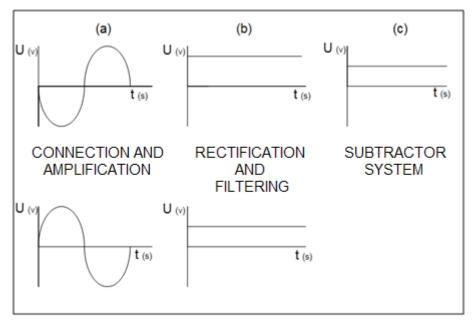
Figure 2. Illustration of the waveforms during the signal conditioning.
