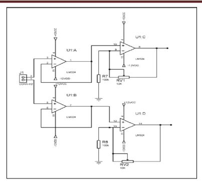
Figure 1. Connection and amplification circuit of the signal conditioning system.
