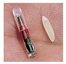
Figure 3 – Chip RFID compared to a grain of rice [14]
