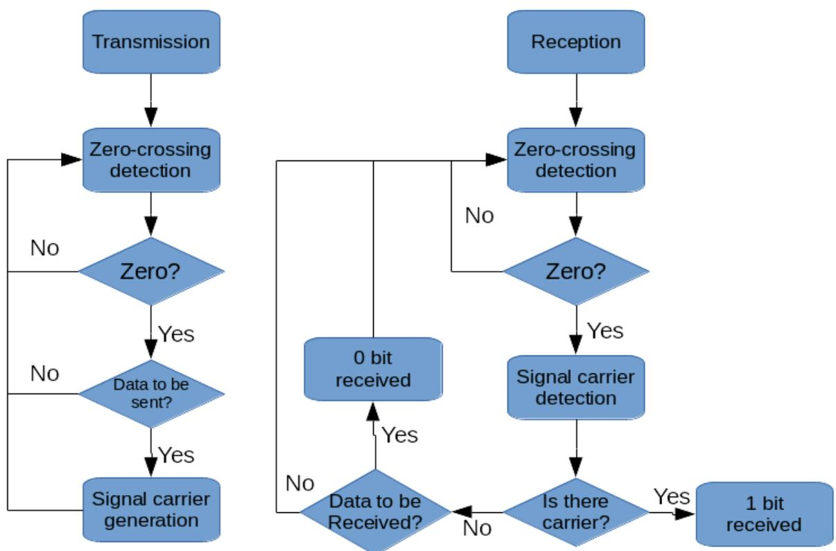
Figure 2: Flowchart of the X10 communication procedure
