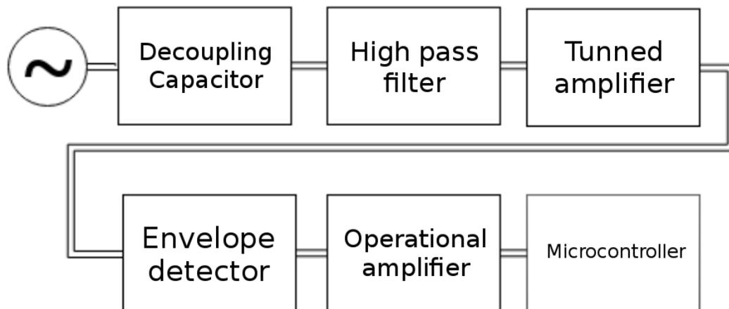
Figure 6: Block diagram of signal carrier detection
