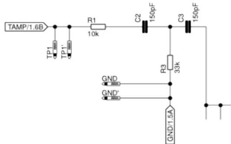
Figure 8: High pass filter circuit
