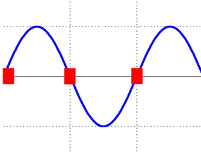
Figure 1: Zero-crossing, where the X10 signal is sent
