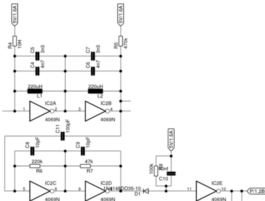
Figure 9: Tuned amplifier and envelope detector
