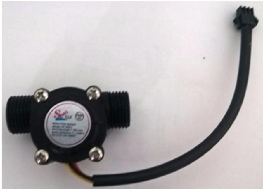
Figure 12: Water flow sensor model YF-S201
