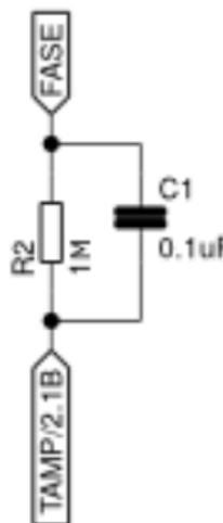
Figure 7: Decoupling capacitor circuit
