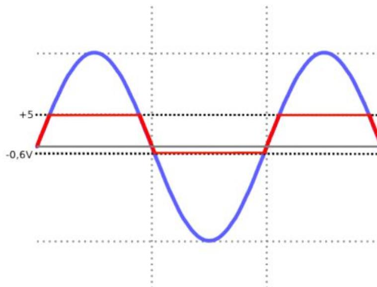
Figure 5: Voltage level present in input pin due to protection circuits
